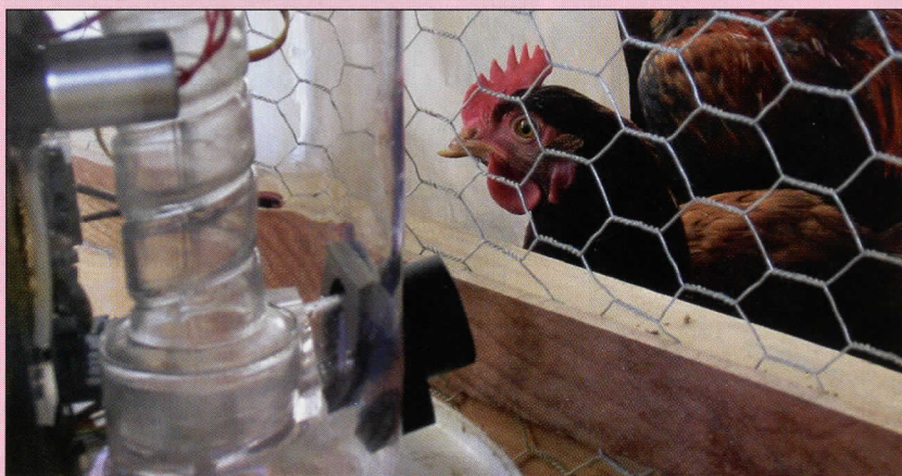
Researchers at the California Animal Health and Food Safety Laboratory and Lawrence Livermore National Laboratory demonstrated that the Newcastle disease virus could be detected using an environmental air sampling system, which is much less labor-intensive and time-consuming than conventional swab sampling.
